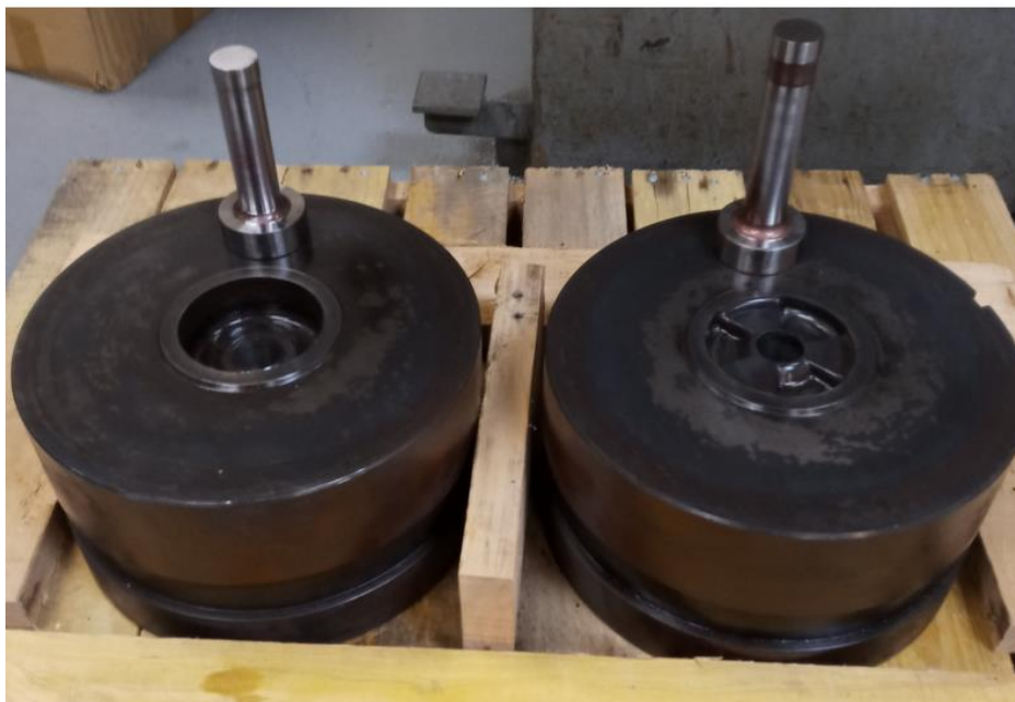
Figure 5.13: Top and bottom preform dies and punches fabricated at NC State University
